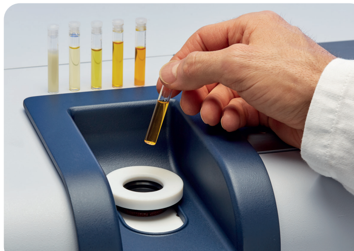
Analysis of liquid products (here oil) in the sample compartment of the MPA II in transmission.
