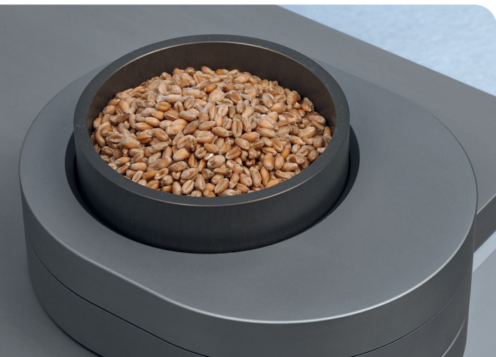
Analysis of solid products (here wheat) on the integrating sphere of the TANGO in diffuse reflection.
