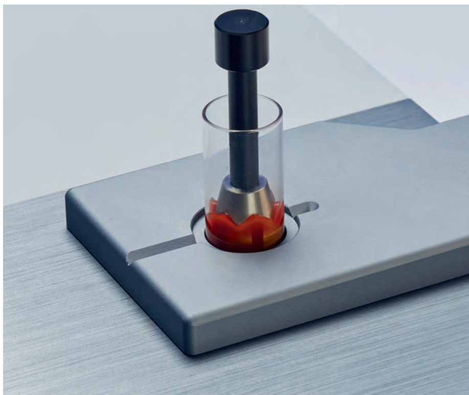
Transflection measurement of ketchup in a 22mm vial on the integrating sphere of the MPA II.
