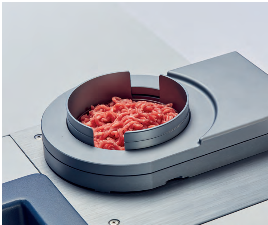
Measurement of minced meat in a polystyrene Petri dish on the integrating sphere of an MPA II spectrometer.
